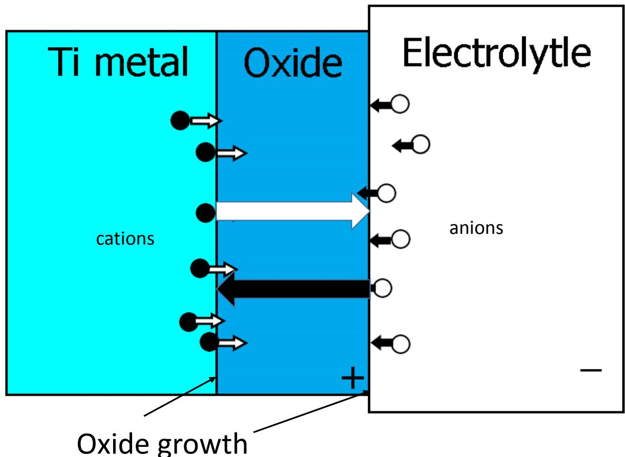
Two major oxide growth mechanism: Point-defect model (PDM) [3]
