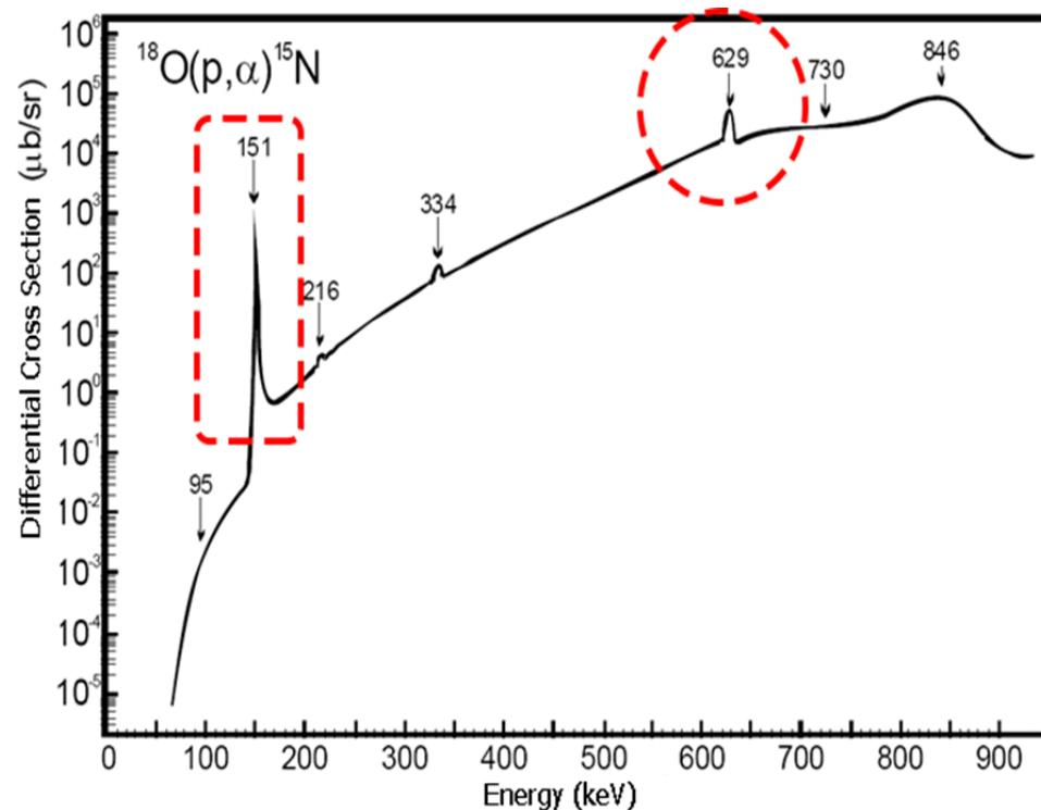
Differential cross sections for the  $^{18}\text{O}$  (p,  $\alpha$ )  $^{15}\text{N}$  reaction. Note the narrow width of 151 keV. DCS decrease by several orders of magnitude [2]
