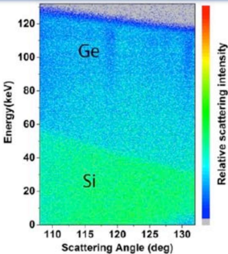
**Fig. 1.** 2D MEIS spectrum measured with 150 keV He<sup>+</sup> projectiles under normal incidence on the SiGe heterostructure grown over crystal Si. The following signals are observed from top to bottom: Ge and Si from the Si<sub>0.7</sub>Ge<sub>0.3</sub>, Si from the substrate. Blocking lines in Ge are also visible.
