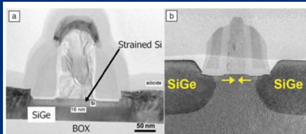
**Figure 1.** (a) Cross-sectional transmission electron microscopy (TEM) image of biaxial (tensile) strained Si *n*-type field-effect transistor (FET) fabricated using SiGe-on-insulator as a growth template. Reprinted with permission from Reference 8. © 2004 American Institute of Physics. (b) Cross-sectional TEM image of an uniaxial strained (compressive) *p*-type FET device using embedded SiGe in the source and drain regions. Reprinted with permission from Reference 10. © 2003 IEEE.
