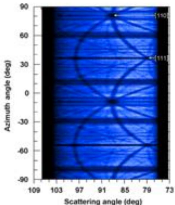
Fig. 3. Cartography of  $\text{He}^+$  ions scattered by the germanium atoms in a SiGe layer to a depth of 18 nm below surface.
