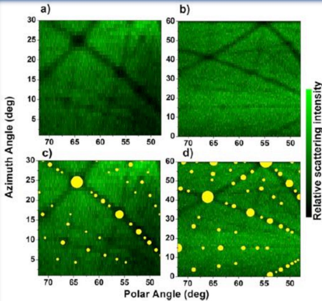
Fig. 6. (a) MEIS cartography of a reference Si (100) sample used for angular calibration. (b) MEIS cartography for  $\text{Si}_{0.8}\text{Ge}_{0.2}$ . (c) and (d) are the same as in (a) and (b) including the main directions represented by circles.
