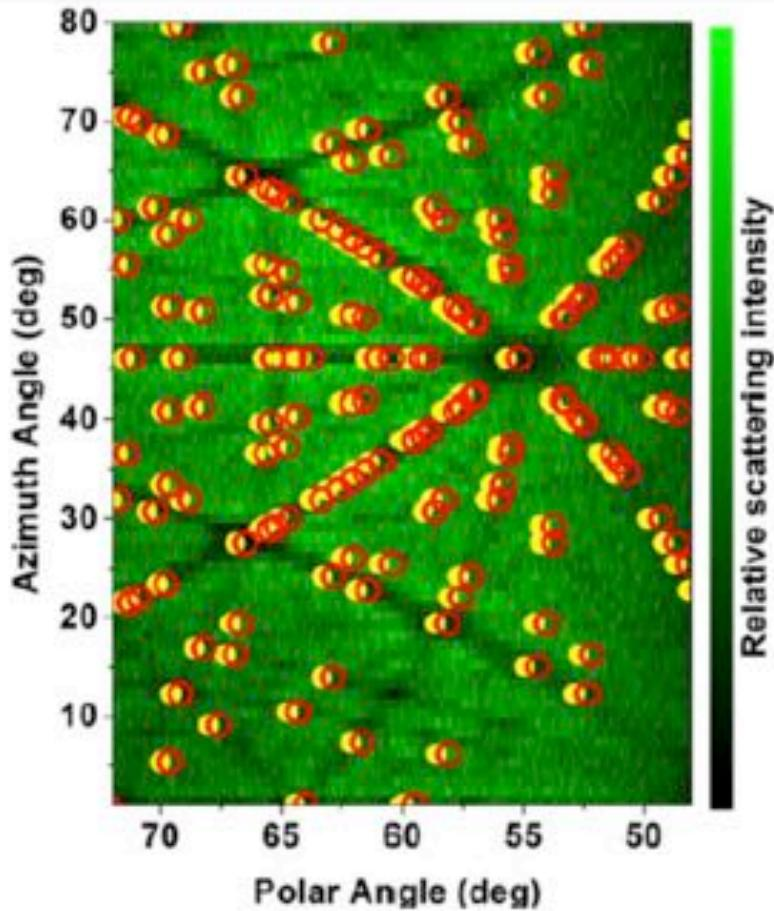
Fig. 4. Cartographic map of a strained-layer  $\text{Si}_{0.7}\text{Ge}_{0.3}/\text{Si}$  using 150 keV  $\text{He}^+$ . Each superimposed circle corresponds to a direction in a relaxed layer (full circles) and 2% uniaxial strain (open circles).
