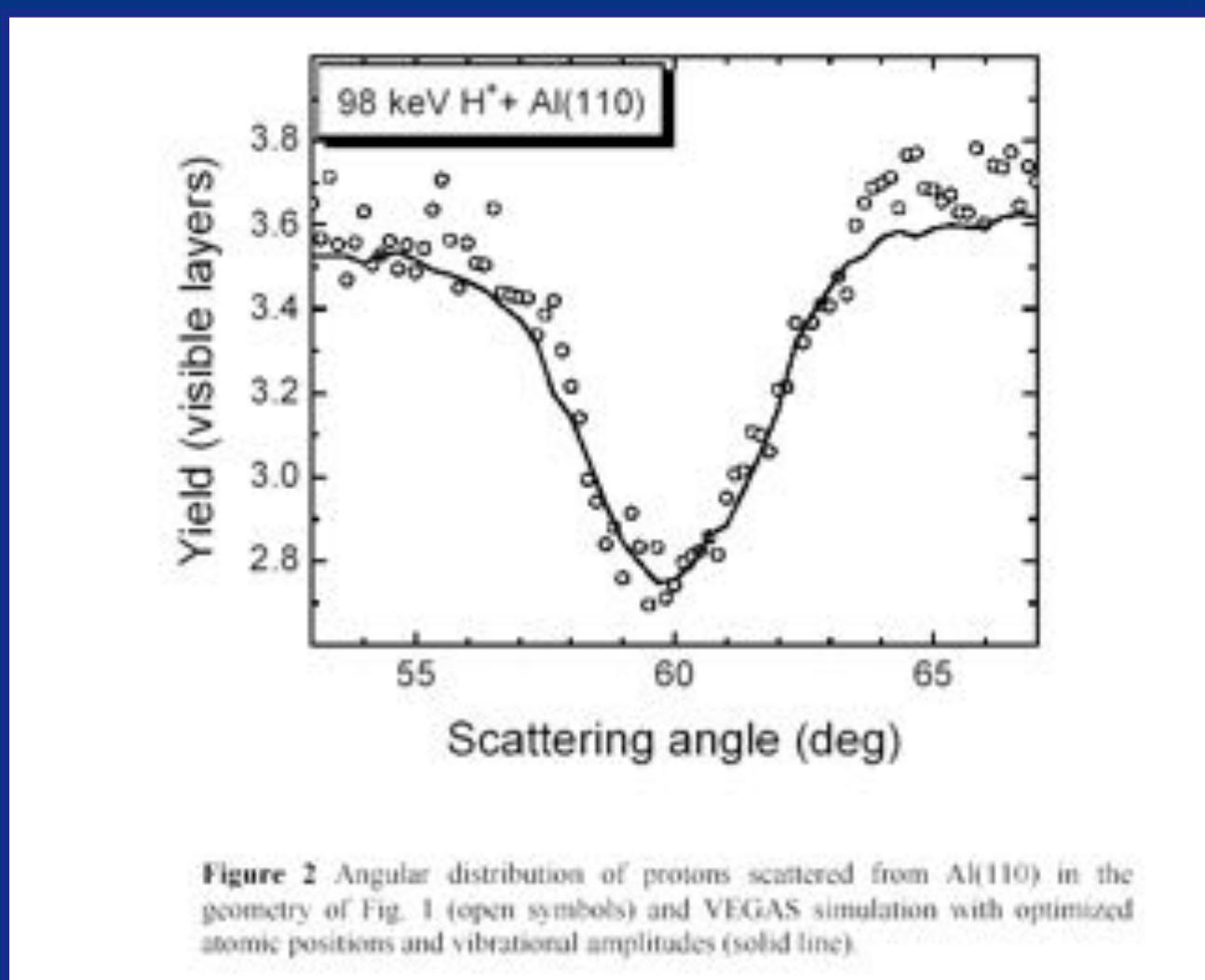
**Figure 2** Angular distribution of protons scattered from Al(110) in the geometry of Fig. 1 (open symbols) and VEGAS simulation with optimized atomic positions and vibrational amplitudes (solid line).
