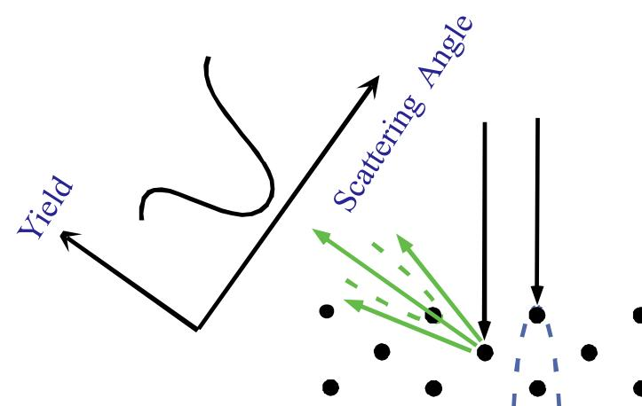
MC ion scattering simulation of angular yield provides **surface structure**.
