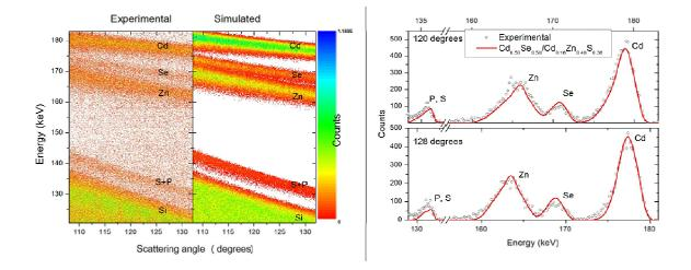
This study shows that the MEIS technique, combined with other analytical techniques, is a powerful method to determine elemental distribution profiles, inside nanoparticles with diameter about 5 nanometers. This allows studies of the formation and stability of the internal structure of QDs when exposed to several kind of processes, like heating and ion irradiation.
